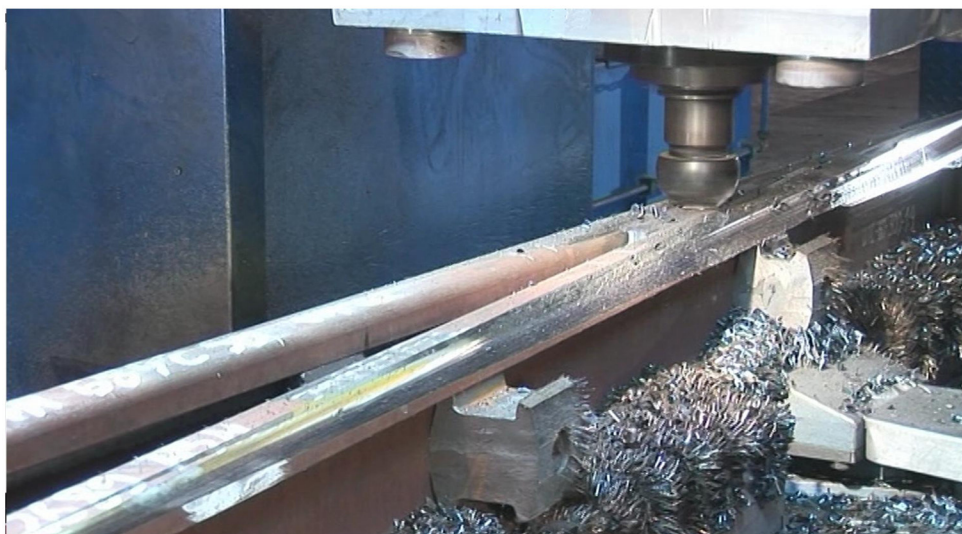
Machining of rails
